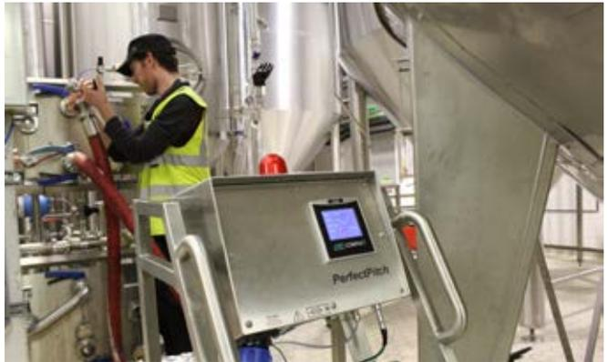
The skid is portable and can be wheeled to the appropriate location within the brewery.
