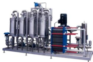
In membrane and column deaeration units O<sub>2</sub> passes from the liquid phase into the gas phase. Vacuum and strip gas on the gas side create a large partial pressure difference. Our special design maximizes the surface for the gas exchange.
