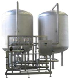
For the reduction of water hardness, anion or cation exchangers are applicable. Mixed bed ion exchangers contain a mixture of anion and cation exchange resins. They are used for simultaneous and highly efficient exchange of both ion types.
